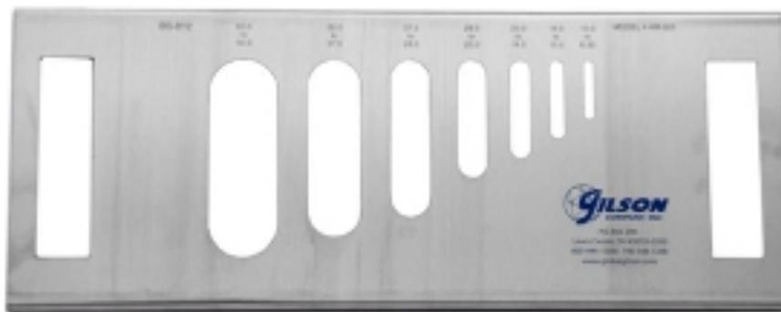
Grid sieves (for flakiness test)
