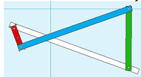
Next the green bar begins to move to the left. As the red bar goes around and around, the green bar goes back and forth. Since the angle through which the green bar turns is only about 25 degrees, the arc of motion is fairly straight. This invites a comparison to the engine. The piston on the engine moves back and forth in exactly a straight line. The top end of the green bar approximates the same motion.
