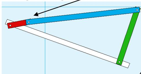
That's because the motion caused by the red bar is at right angles to the blue bar. At that instant, the blue bar is rotating about its joint at the end where it attaches to the green bar.
