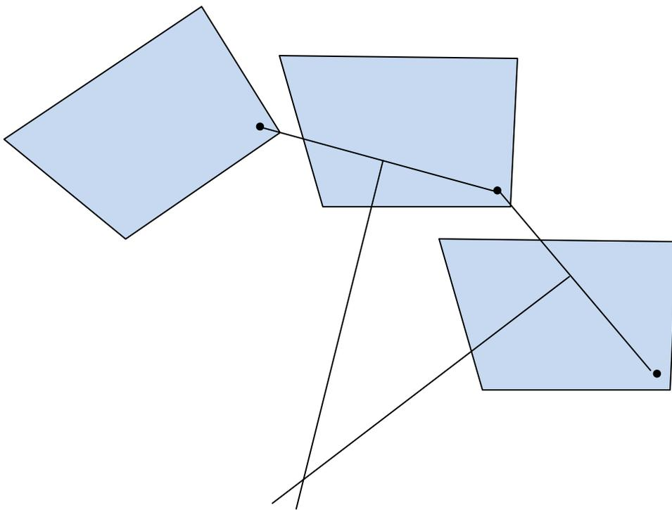
Now, you can do the same thing for the other side of the mechanism. On the left side we have a point we chose to connect the bar to the container. Move the container through its three desired positions and we get three desired points. Draw lines, bisect the segments, form perpendicular lines, and find their intersection. Now you have the fourth bar in your mechanism.
